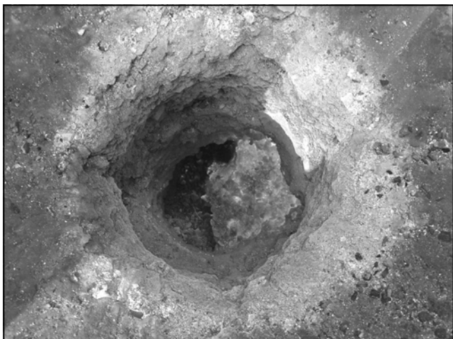
Looking down at the very hot bloom in the furnace; the tuyere is to the right
